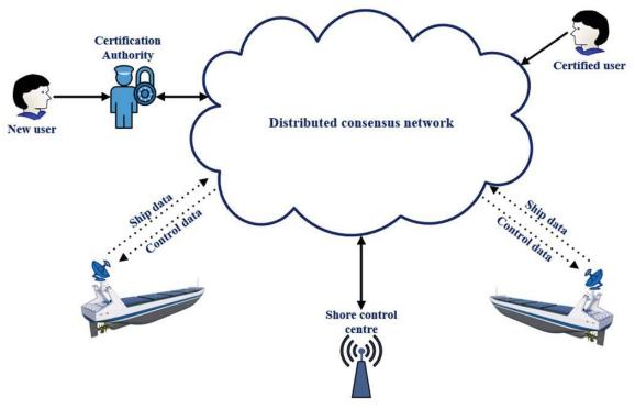
Figure 2: Proposed usage of the BT for autonomous vessels control Source: Authors
